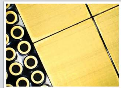
Isolated planes on back can be used for ground or power
